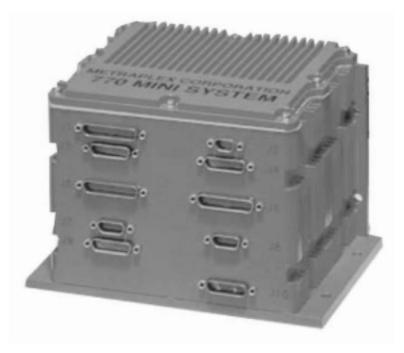
Specially designed for tight spaces and severe environments, Miniature Encoders are ideal for flight testing civilian and military aircraft, as well as mobile ground based data acquisition. The 770 PCM System housings are designed to provide maximum accuracy of test results. All housings are environmentally sealed with EMI/RFI shielding and gasketing. Microminiature D-type Metal (MDM) connectors provide hermetic seals and electromagnetic shields for signal wires and cables.
